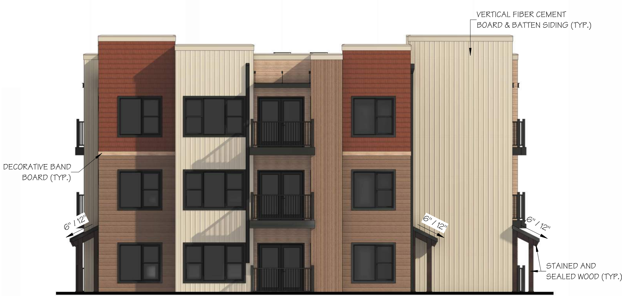
2 AP6 BUILDING #1 LEFT SIDE ELEVATION SCALE: 1/8" = 1'-0"
