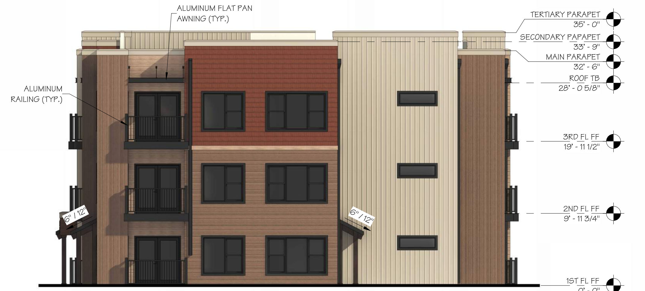
3 AP7 BUILDING #2 RIGHT SIDE ELEVATION SCALE: 1/8" = 1'-0"
