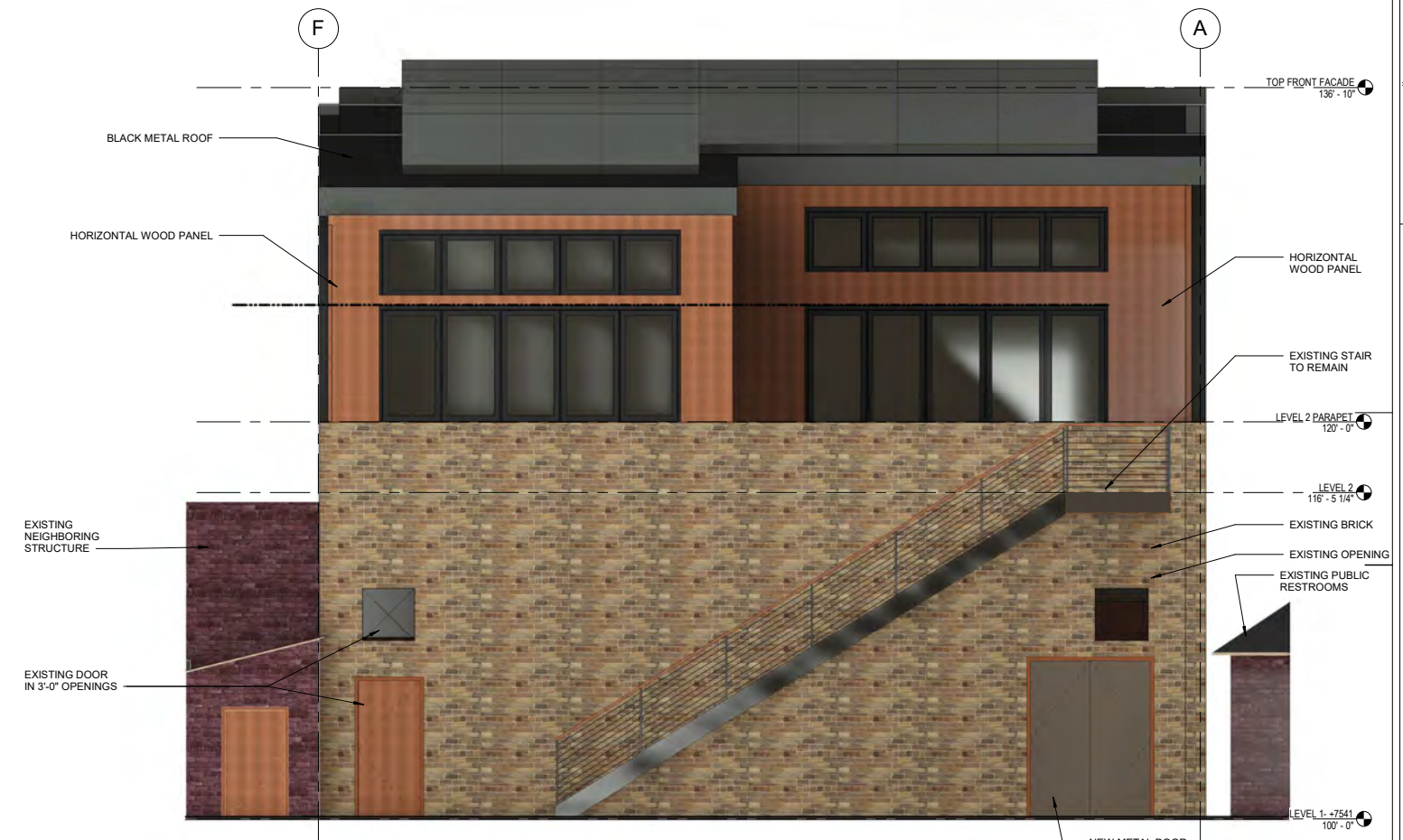
1 South Exterior Elevation 1/4" = 1'-0"
