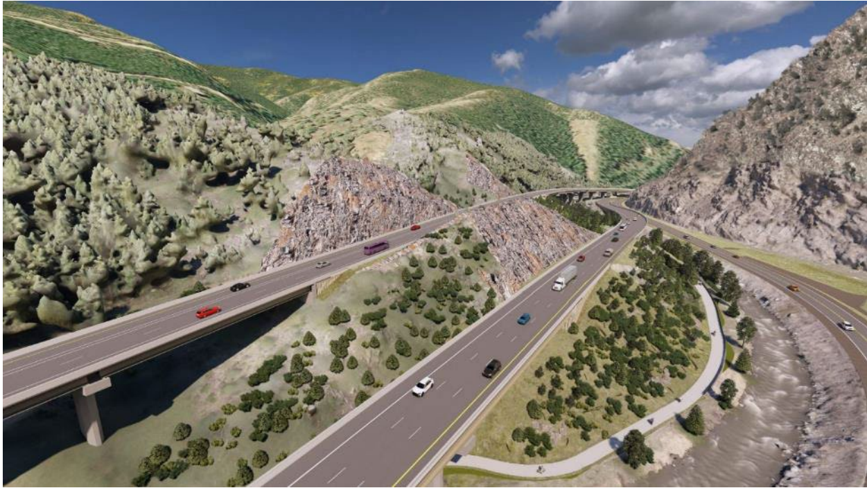
Figure 5. Vertical alignment of I-70 through the “saddle cut” lowers the elevated eastbound section compared to the EA Preferred Alternative
