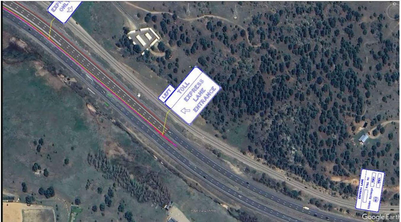
Figure 3 Express Lane Entrance (ingress transition shown in figure between toll sign and double white line)
