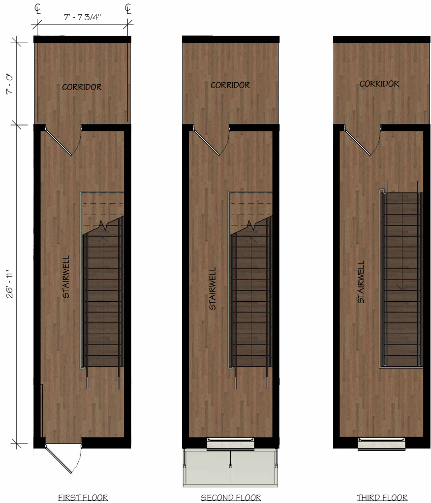
TYP. STAIRWELL FLOOR PLANS
