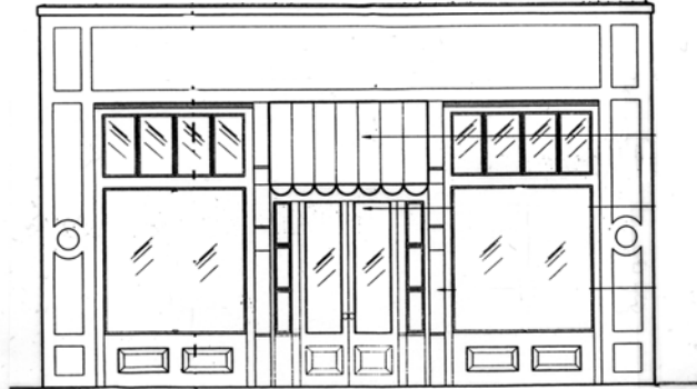
Inappropriate entrance design.
